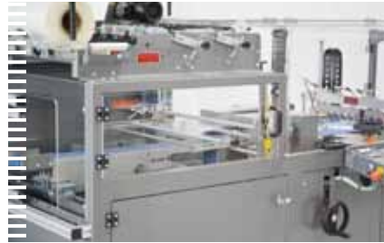
The Servo Packer 500: Wrapping products at speed, whether in film or paper.
