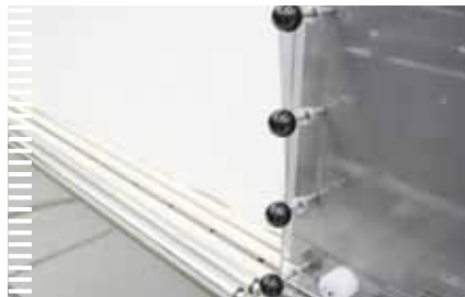
Easily adjustable shift register for adaptation to the product outline.
