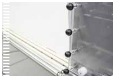
Easily adjustable shift register for adaptation to the product outline.
