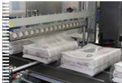
Super Wrap 500: Especially designed for sleevewrapping in PE-film.
