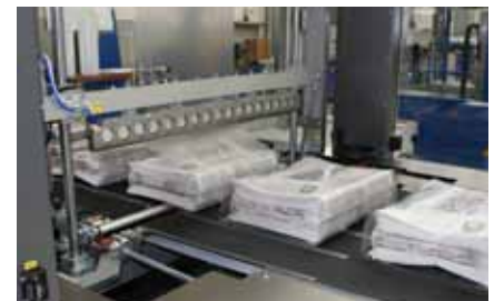
The special feature of the Super Wrap Servo: Reliably packaging in continuous motion.
