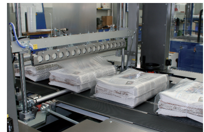
The special feature of the Super Wrap Servo: Reliably packaging in continuous motion.
