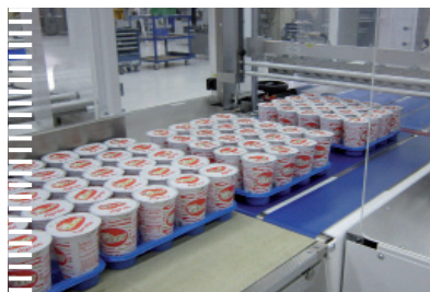
The special feature of the Super Wrap Servo: Reliably packaging in continuous motion.
