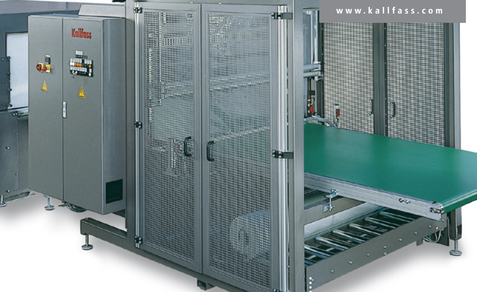
Large-format sleeve wrapper with shrink tunnel
