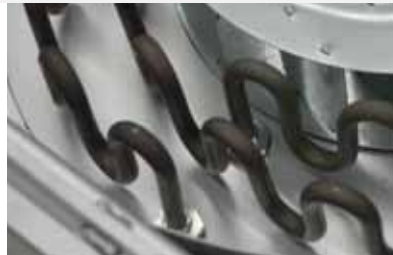
The ring nozzle heating system provides constantly uniform heat energy transfer into the shrink film.
