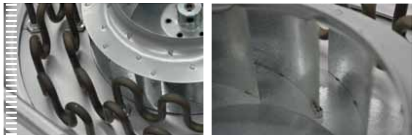
The ring nozzle heating system provide uniform heat transfer into the shrink film.
