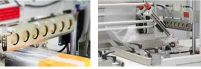
The transverse seal bar is only 350 mm long. Easily adjustable forming shoe, in both horizontal and vertikal direction. The product feed is perpendicular to the flow direction.
