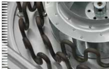
The ring nozzle heating system provide uniform heat transfer into the shrink film.
